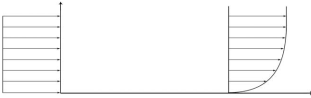
Fig. 11. The formation of a boundary layer next to a wall (horizontal thick black line). The y-axis represents the relative distance away from the wall. The set of arrows on the left and right represent the velocity profiles at different distances from the wall; the length of the arrow is proportional to the magnitude of the velocity. The arrows indicate the flow is going in a left to right direction. The velocity is uniform on the left because those points are not adjacent to the wall. The velocity at the wall is zero, and the velocity profile on the right represents the boundary layer. (See text for further details.)
